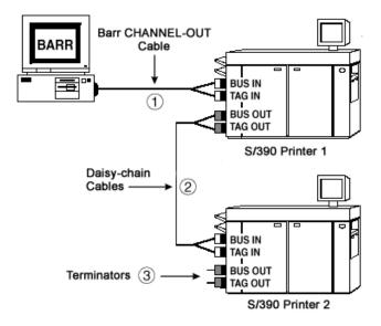
Daisy chain printers using Bus & Tag cables.
