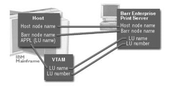
Parameters used when configuring BARR/NJE for a Barr SNA connection. Use the same information in all phases for configuring BARR/NJE.
