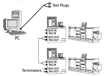
Connect one end of the cable to the adapter and the other end to the test plugs.
