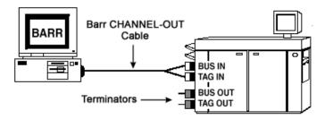
Attach the printer to the computer. If you have only one printer, also attach terminator plugs.
