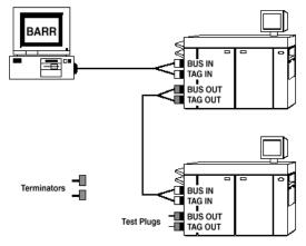
Remove the terminators and install the test plugs.
