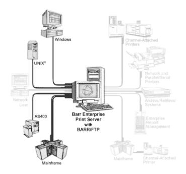
To upload files to a host computer, BARR/FTP uses the FTP put command to 'put' files into a pre-configured location on an FTP server or host computer. The FTP output device is configured as a spool printer in the Spool Window.
