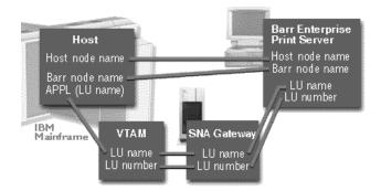
Parameters used when configuring BARR/NJE for an SNA connection. Use the same information in all phases of configuring BARR/NJE.
