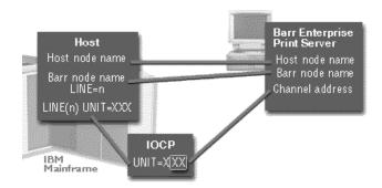
Parameters used when configuring BARR/NJE for a CTC connection. Use the same information in all phases for configuring BARR/NJE.
