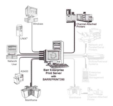
BARR/PRINT390 integrates easily into the Windows print architecture. The module is implemented with two components: a Barr PRINT390 printer driver and a Barr PRINT390 port monitor. The Barr PRINT390 printer driver prepares data for a channel printer by generating EBCDIC data with S/390 machine carriage control. The Barr PRINT390 port monitor is used to communicate with the CHANNEL-OUT adapter.
